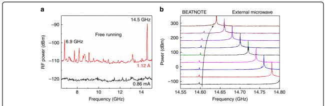
**Fig. 2 Beatnote and injection locking at the harmonic frequency. a** RF spectrum collected with the QCL on and no RF injection, showing strong beatnotes at the fundamental (6.9GHz) and second harmonic (14.5GHz) round-trip frequencies. **b** RF injection locking of the second harmonic beatnote with the external microwave modulation (power: 16dBm) brought closer in frequency to that of the beatnote (The spectra have been offset for clarity.)
