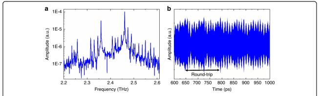
**Fig. 4 Self-starting high-harmonic emission.** a Free-running QCL spectrum showing several frequency bands separated by 100GHz corresponding to the 15th harmonic of the round-trip frequency. Each frequency band has a mode spacing corresponding to the second harmonic of the round-trip frequency. **b** Time-resolved electric field profiles with multiple pulses per round trip and an 'over-modulation' at half the round-trip time
