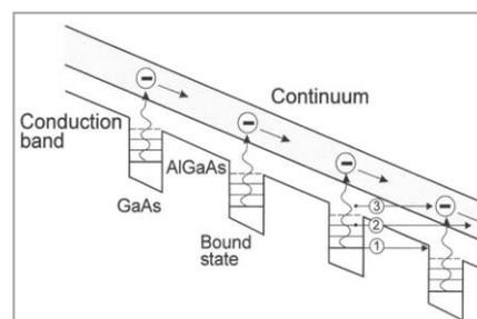
In this context, the project's main goal is to study on a model system how virtual photons – i.e. the sole presence of a cavity – affect its energy levels of and therefore its electronic properties. The model system we will use is a semiconductor quantum heterostructure consisting in a periodic stack of doped quantum wells, operating in the dark and at cryogenic temperatures to ensure that no external photonic or thermal excitation perturbs the system.
